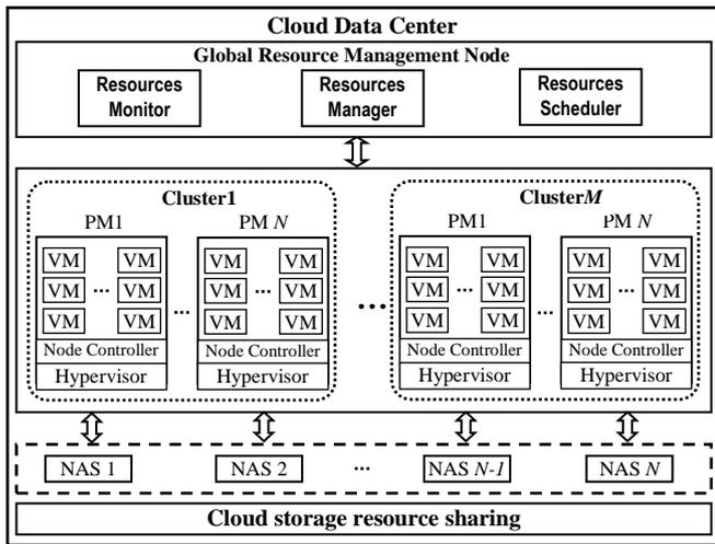
Fig. 1. Virtual Resource Model of Data Center [4]
