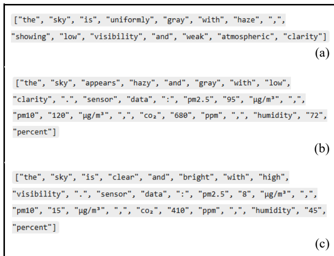
Fig. 3 sample VLM output (a) using Fig. 2 sample without hardware sensor measurement (b) using Fig. 2 sample with hardware sensor measurement © using a good sample with hardware sensor measurement
